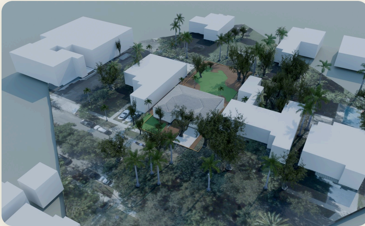
A test property built in 3D by our own scripts from the laser survey and our measurements. Local render.
